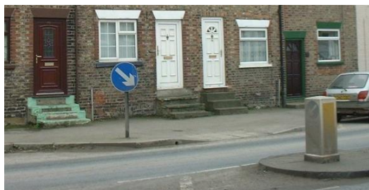
Figure 1 Signs should be appropriately sized and used in the right location – a keep right sign wrongly used as there is no possibility of keeping left of it
