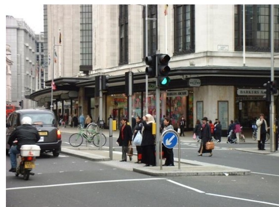
Figure 8 Staggered pedestrian crossing without a guard rail
