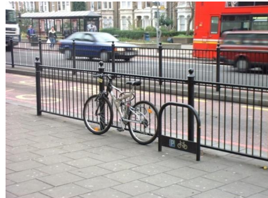
Figure 1 Double lines of guard rails around a bus lane– the nearer being used as a cycle rack
