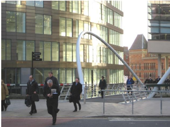
Figure 9 Pedestrian priority shown with uncontrolled crossing on the desire line
