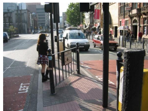
Figure 3 Guard rails poorly sited or over installed can alienate pedestrians
